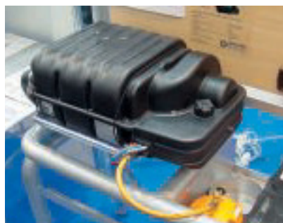
Energie-Transfer: Self-Energy EG 20 von Reimo verwandelt Gas in Strom.
